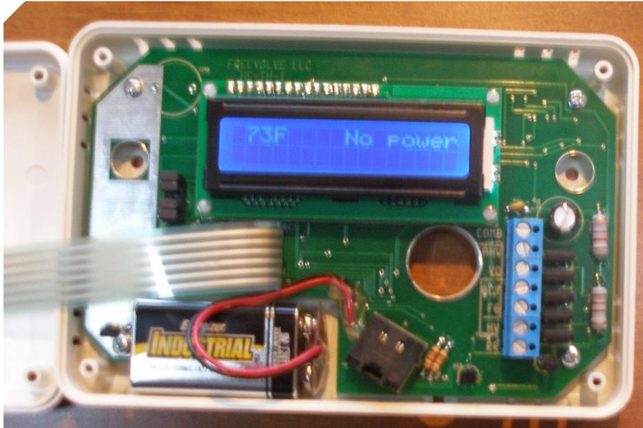
The Thermostat Module will go through a brief startup procedure, then the display will show the current temperature with a “No power” indicator in the upper right side.
