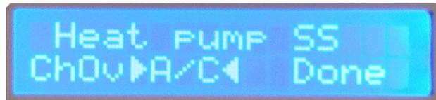
The system sets the active changeover valve state to AC. When finished, navigate to “Done” and press Select. The system will return to the main screen and the Thermostat Module is now configured to work with a single-stage heat-pump HVAC system.
